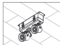
Ceiling (Type C) (Installation without accessories)
